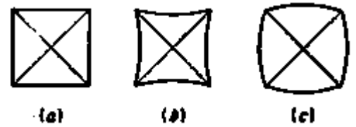
a. perfect indentation b. pincushion indentation due to sinking in c. barreled indentation due to ridging.
