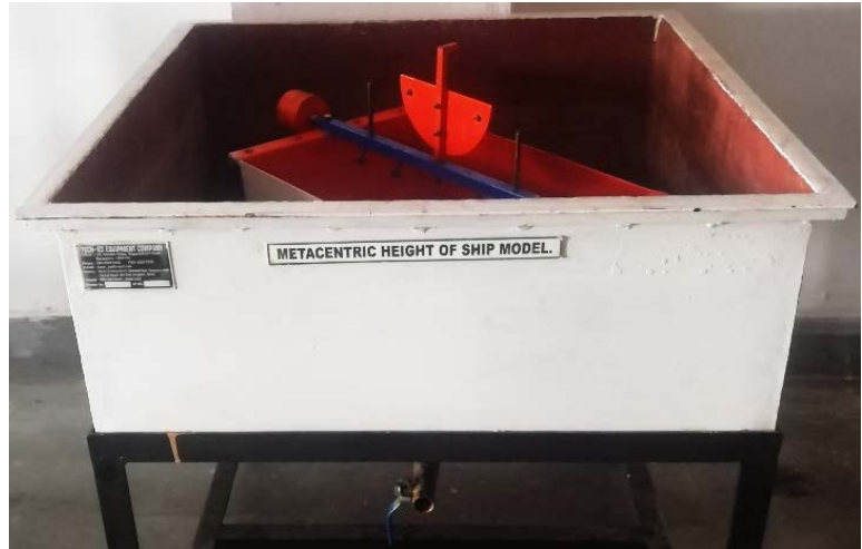
Fig. 1.1. Experimental set up of metacentric height apparatus.
