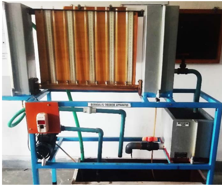
Fig. 2.1. Experimental set up of Bernoulli's theorem apparatus.
