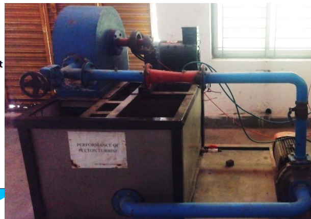
Fig. 11.1. Pelton wheel experimental setup
