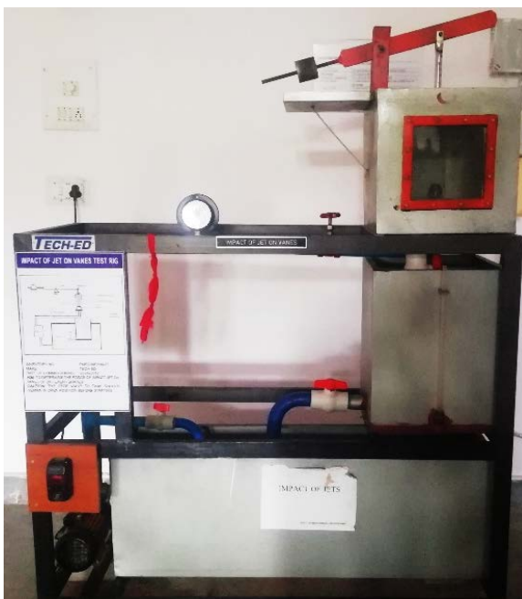
Fig. 10.1. Experimental setup of Impact of jet apparatus.
