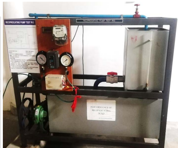
Fig. 15.1 Schematic diagram of Reciprocating pump
